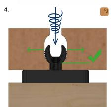
Application of SFIX Clips for the installation of wall covering
