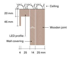
Made of two pieces. Same finishing as of the wall panel.
